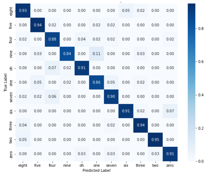
Figure 4. Confusion matrix of multiclass classification using a combined CNN-LSTM model in noisy speech (Aurora2 dataset).
